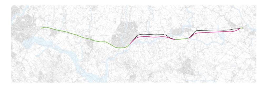
**Option 3** would widen the existing A12 corridor between junctions 19-22 to three lanes in each direction. At junction 22, it leaves the existing corridor and creates a new 3 lane bypass to the south running in parallel with the existing A12 until junction 23 where it would re-join the current corridor. It then follows the existing A12 corridor between junction 23-25 which would widen to three lanes in each direction
