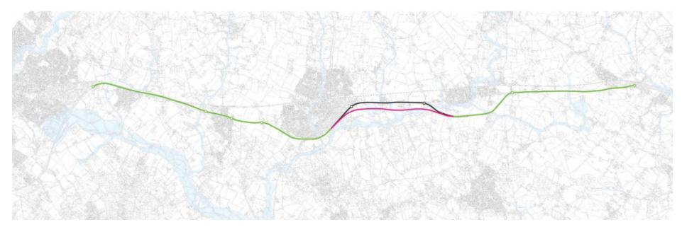
**Option 4** would widen the existing A12 corridor between junctions 19-24 to three lanes in each direction as with Option 1. At junction 24 it leaves the existing corridor and creates a new 3 lane bypass to the south, running in parallel with the existing A12 until junction 25 where it would re-join the current corridor.
