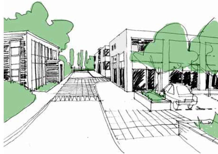
ABOVE: The main vehicular access into the development follows the existing access way to the playing fields. Raised tables at junctions and main pedestrian crossing points calm traffic.
