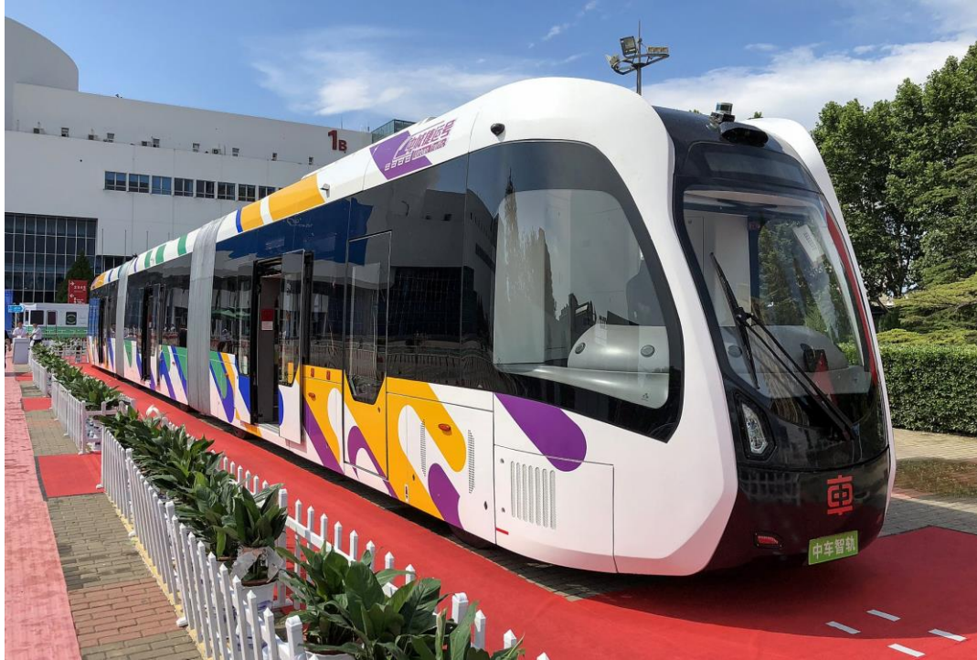
Figure 2-3: “Trackless trains” – self-driving vehicles, which have the rubber-wheels of a bus, use sensor technology to follow markings painted on the streets. Source: Wikimedia Commons 3
