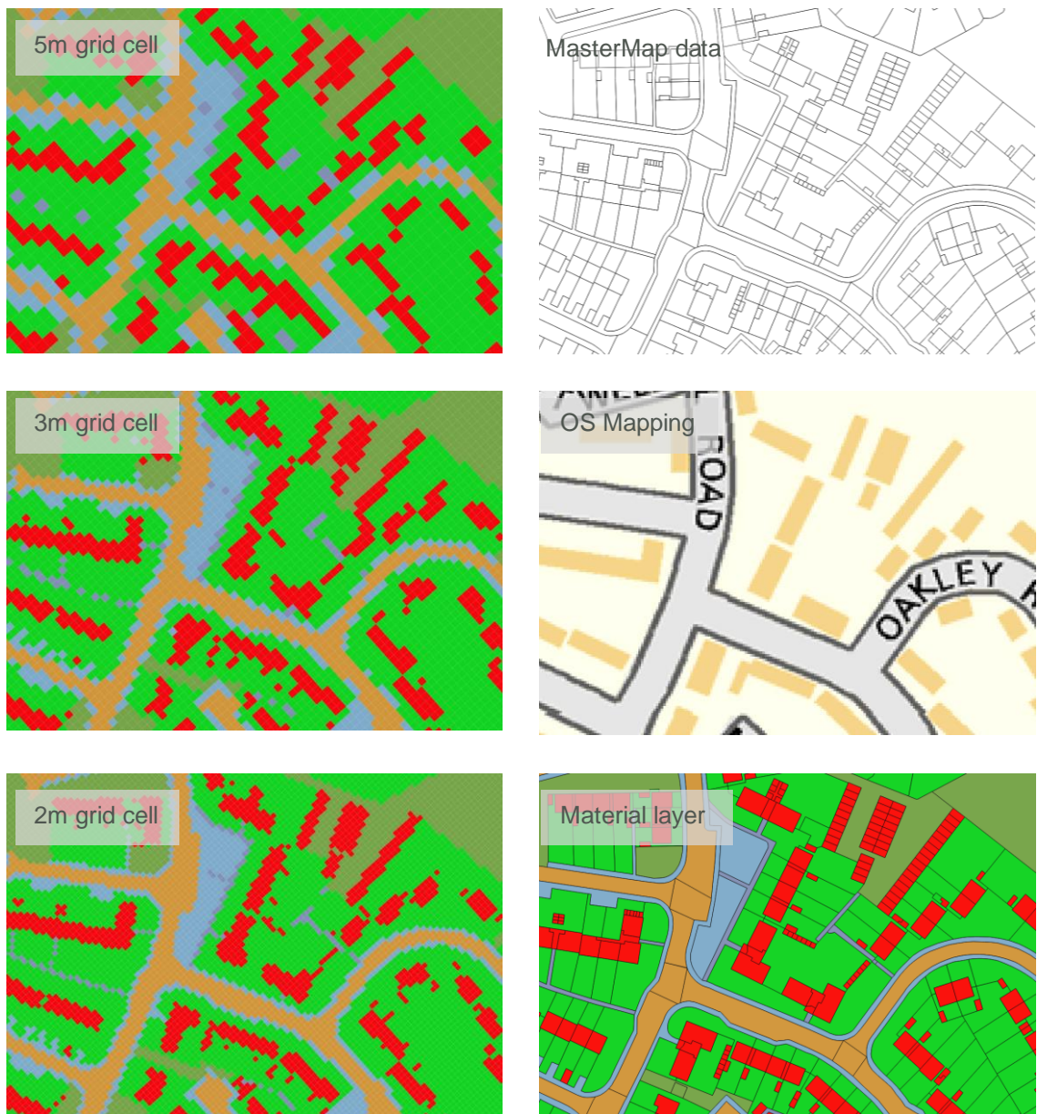
Figure 4-3 Cell size resolution difference
