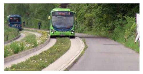
Cambridge Guided Busway - an example of the type of solution that could be implemented on the Flitch line. Operational since 2011 it runs for 25km and connects Cambridge to Huntingdon (60min) and Trumpington (15min). It runs at a 7 minute frequency and reaches speeds of 90kph. Image Source: Google
