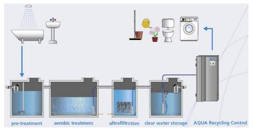
Combined rainwater harvesting and greywater recycling systems can be particularly effective, with the use of rainwater supplementing greywater flows at peak demand times (e.g. morning and evenings).
