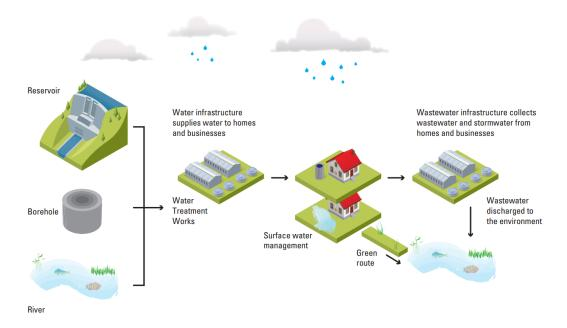
A broad overview of the water cycle and the role of water and wastewater infrastructure within the cycle is illustrated in Figure 3. Wastewater is generally produced following the use of potable water in homes, businesses, industrial processes and in certain areas can include surface water runoff.
