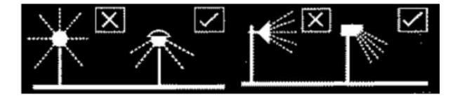
(c) Lighting should be designed to the correct standard for the task and should not over-light. (See Appendix 2, *Relevant Publications for Standards for Lighting*). Over-lighting is a cause of obtrusive light and also represents a waste of money and energy.
