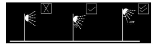
(e) Lighting should be directed to minimise and preferably avoid light spillage onto neighbouring properties. Wherever possible use floodlights with asymmetric beams that permit the front glazing to be kept at or near parallel to the surface being lit.
